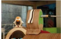
From this perspective, we can see the track on which the tweeter slides. We can also identify the wooden case structure. Here too multilayer birch wood is used.
